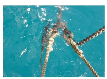
If you anchor on a chain rode, you should always use some nylon rope as a snubber to absorb shock loads from the chain that would otherwise be carried directly by the boat and its hardware. Be sure to use three-strand nylon rope for maximum stretch. It's also a good idea to use two separate lines, effectively creating a snubber bridle.
