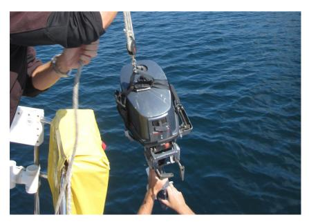
It's always tricky lifting out board engines onto a boat with a high freeboard. We used a short length of high-modulus Amsteel rope to create a lifting strap that we could loop through the fitting on the end of the boom. We then put a snap shackle on this strap and made up a 3:1 tackle with a fiddle block and cam cleat on one end and a becket block with another snap shackle on the other.
