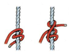
Wrap a line twice around another fixed line or post. Take a third turn by passing the working end of the first line over its standing end and then around the second line above the first two turns. Pull on the standing part of the first line and the hitch will not slip down the second line.
