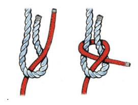
Form a bight in the end of one line. Pass the end of the other line through the bight from beneath and around behind both parts of the first line. Finish the knot by passing the working end of the second line under itself, and then pull the knot tight.
