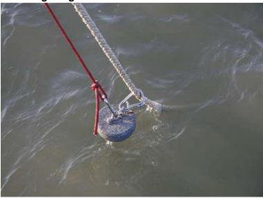
Anchor chums or angels are heavy weights, often lead, that are lowered down the anchor rode after you have anchored
