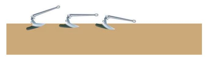
With a fluke-type anchor, it's easy to illustrate the effect of increasing scope on the holding power of an anchor: more is clearly better!
