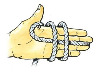
To keep a line from pulling through a block or rope clutch, a knot should be tied in the end of it. The most secure knot for doing this is the double overhand stopper knot, known as the stopper knot for short. Unlike a simple overhand knot or a figure eight knot, this knot does not come loose easily.
