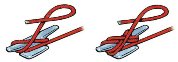
Walk down a dock in any marina and you will see many dock lines improperly secured to cleats. A proper cleat hitch is easy to tie, very effective and it can be released under load without worrying about losing a finger in the process. Any time you make off a line on a cleat, on a dock or on deck, this is the knot to use.
