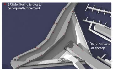
The Sketch shows two bunds making a triangle from the Railway Jetty to the East Pier to create a dry area to complete the works to the Railway Jetty and the inner side of the East Pier wall.
